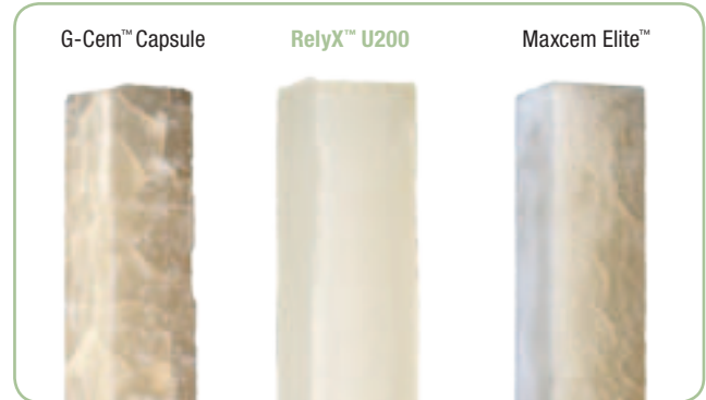
Fig. 7: Results of stress test on self-adhesive resin cements. All samples were self-cured and thermocycled 10,000 times. Source: 3M ESPE internal data
